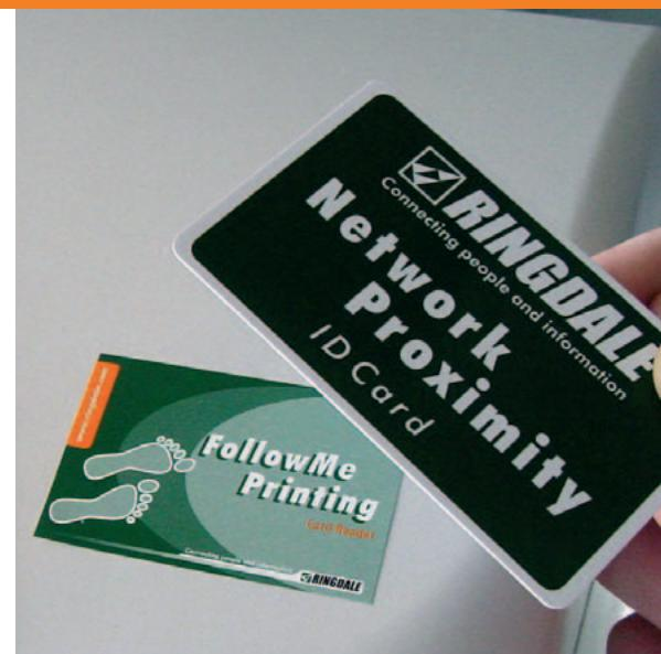
At the printer, JetCAPS FollowMe printing uses numeric PIN codes, fingerprints, barcodes, proximity or swipe cards to identify the user and release the print job or to enable the copier functionality. Messages on the front panel inform users about their credit (quota) level, print job status or access rights, as appropriate.
