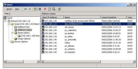
Look for the J-Box suffix followed by the box's MAC address. In case you don't have the DHCP address, use the PING/ARP procedure to discover the box's IP.
