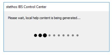
The IBS CC build in online help requires a permanent internet access. Sometimes the installation is performed from a service notebook without internet access, as the customer might not grant access to the internet. If IBS CC recognizes that no online access is possible then it uses a build-in copy of the online help which might not
